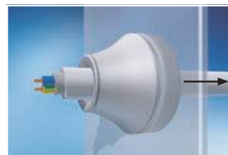
将电缆向后拉一厘米, 电缆密封环就被锁在固定位置 The grommet is the locked in position by pulling it back about a centimetre
